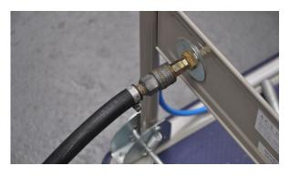
Adjust the pressure to the pump at approx. 4 bar. (1) and the spray pressure to the gun at 5.0 bar. (2)
